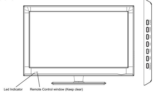
(IR) Infrared Receiver: Receives IR signals from the remote control. (Power on/Standby)LED Indicator: Press POWER to turn on and off.
